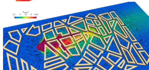
Figure 6. Fields of instantaneous (a) streamwise velocity and (b) concentration in horizontal slice at 1.8 m
