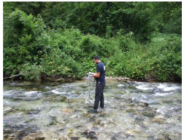
Figure 12. Flow measurement using a flow-tracer
