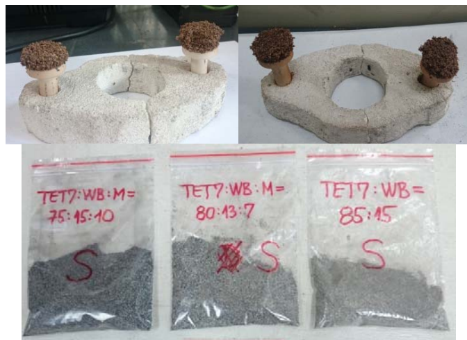
Figure 6. Samples of deposits of ash from the furnace and slag at the exit from the furnace during the co-firing of LC lignite with different types and content of biomass in the mixture – see also [9] and [25]
