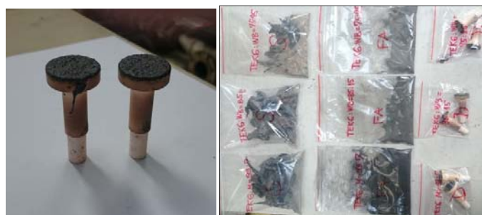
Figure 10. Samples of deposits and slag during co-firing of biomass with coal BC - see also [22]
