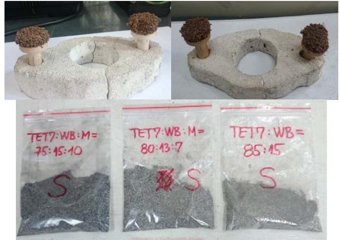
**Figure 6.** Samples of deposits of ash from the furnace and slag at the exit from the furnace during the co-firing of LC lignite with different types and content of biomass in the mixture – see also [9] and [25]
