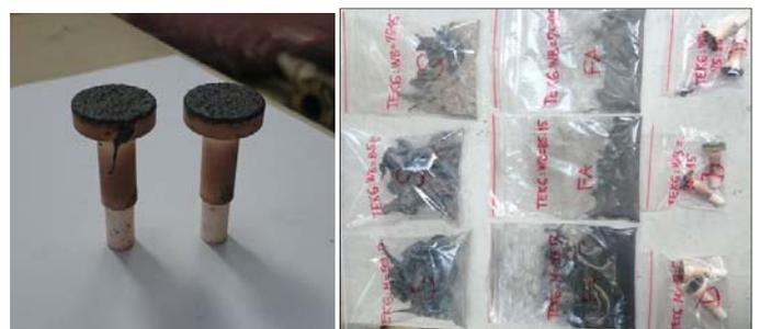
**Figure 10.** Samples of deposits and slag during co-firing of biomass with coal BC - see also [22]
