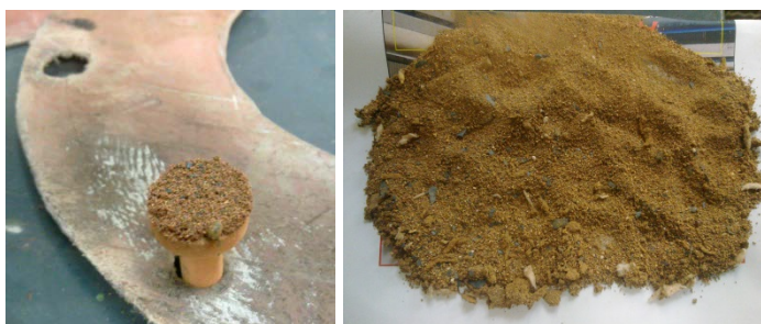
Figure 6. Basic test mode settings: UB(95)P5, 1400^\circ\text{C} , \lambda_1/\lambda=0.95/1.15 ; ash deposit on ceramic tablet - left, slag from reactor bottom/furnace - right
