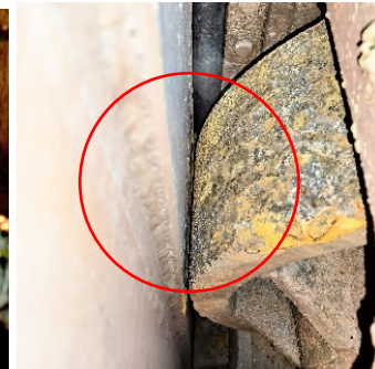
Figure 4. Wheel not in contact with wheel track
