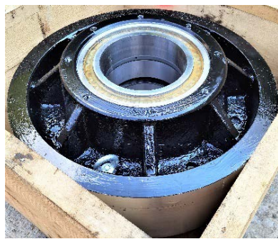
Figure 9. Refurbished wheel with welded stainless steel and packed with roller bearings
