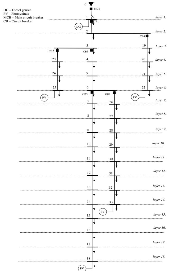
Figure 3. Microgrid testbed
