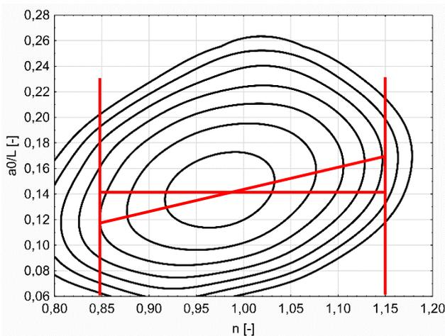
**Figure 9.** Influence of blades relative opening to their length on operating range expansion at different rotational speeds
