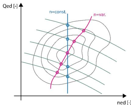
**Figure 1.** Variable speed operated turbine – example [5]
