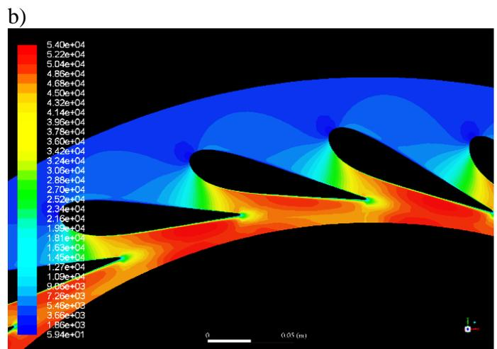
**Figure 13.** Dynamic pressure contours a) (Developed Model 1), b) (Francis 99 Guide vanes)
