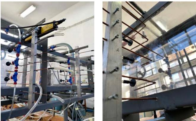
**Figure 1.** Experimental system for measurement of velocity: rectangular conduit with measuring sections and equipment
