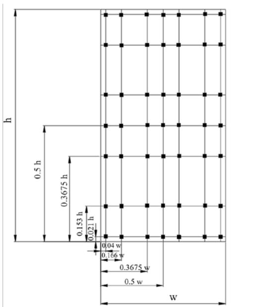
Figure 2. Measuring points in the conduit cross-section
