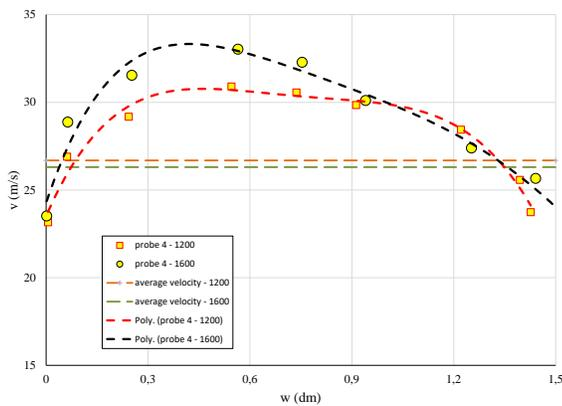
**Figure 12.** Velocity profile and average velocity at 1200 mm and 1600 mm conduit length
