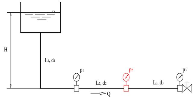
**Figure 4.** Pipeline with serial connection of branches (Case 4)
