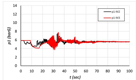
b) pipeline of different wall material at parallel branches (M2 &M3)
